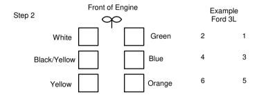
Write the cylinder layout of your engine in the blocks above. Make sure which side is the No1 cylinder and how they are numbered on your engine. Then write the corresponding colour of each cylinder next to your coil number on the lines marked X on the drawing. This will ensure that the sequence of spark is correct.
